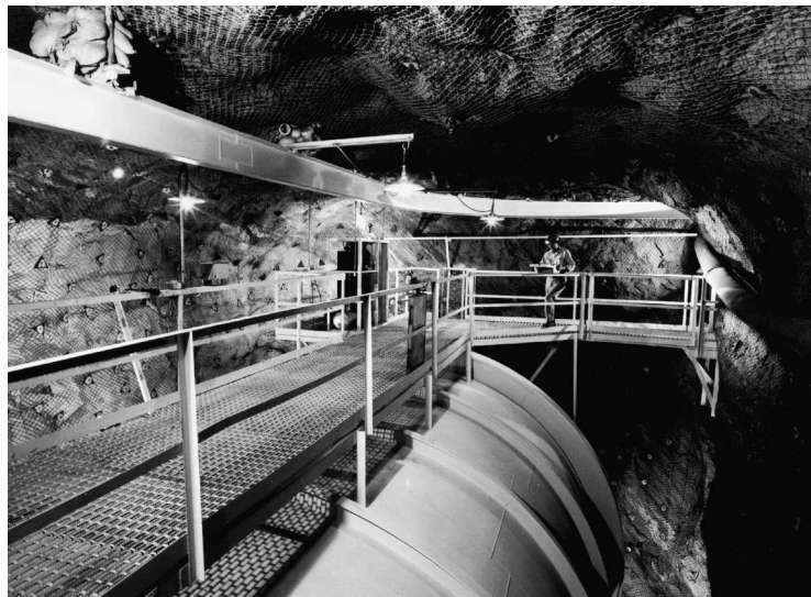
FIGURE 8 Raymond Davis's solar neutrino detector. The tank was located 1478 m (4850 ft) below ground in the Homestake Gold Mine in Lead, South Dakota, and was filled with 615,000 kg of \text{C}_2\text{Cl}_4 in a volume of 377,000 liters (100,000 gallons). (Courtesy of Brookhaven National Laboratory.)
